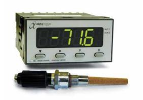
The dewTEC Model DS2000 from Alpha Moisture Systems is a single channel, online hygrometer designed to accurately measure dewpoint in process gases and dry compressed air. This panel mounted DIN style dewpoint meter combines advanced digital technology with the industry leading ultra high capacitance aluminium oxide sensors - the acknowledged industry benchmark for trace moisture measurement in process gases.
