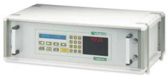
The Model 542 is a versatile, programmable gas analyser, based on the principles of thermal conductivity, capable of measuring almost any combination of gases. The instrument is especially suitable for measurements of mixtures containing hydrogen or helium.
