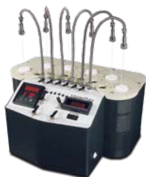
The MasterPrep Degasser set up for vacuum degassing
